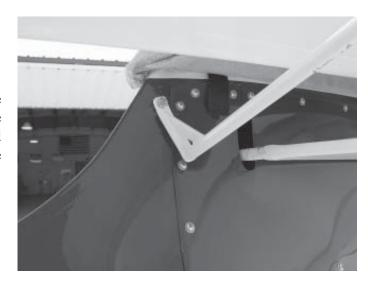
Attach each tow brace to the front spars, as shown.
