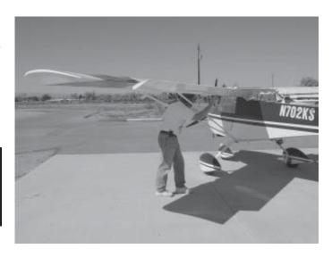
By the time the wing is fully folded, the flaperon must be oriented vertically to keep from being damaged by the vertical stabilizer.
