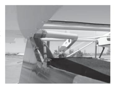
Remove the hardware that holds the fairings to the root of the leading edge of the wings. Place the fairings in a safe place.
