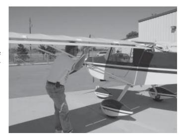
Continue to swing the wing slowly rearward while rotating the trailing edge of the flaperon upward.
