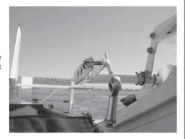
Move the push-pull tube so that it is out of the way of the flaperon horn. As the wing is pivoted about the rear spar attachment point, the push-pull tube must not catch on the horn. Also push any available slack in the fuel lines going to the wing tank (if installed) through the opening in the rear of the butt rib.
