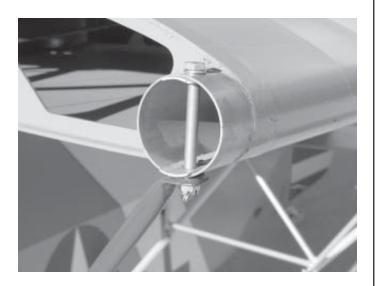
Connect the lower end of each tow brace to the front ear of the lift strut attachment on the fuselage carry-through tube.
