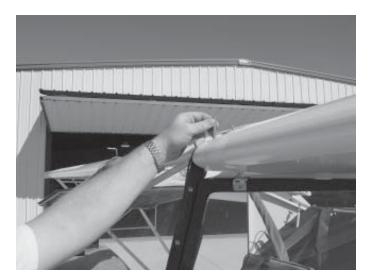
While holding the jury strut with one hand, remove the pin from the spar with your other hand.
