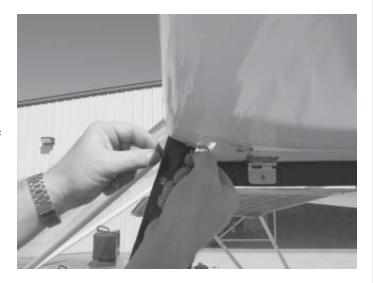
Push the clevis pin up through the front spar. Leave the pin in the top hole of the spar so the wing cannot swing.
